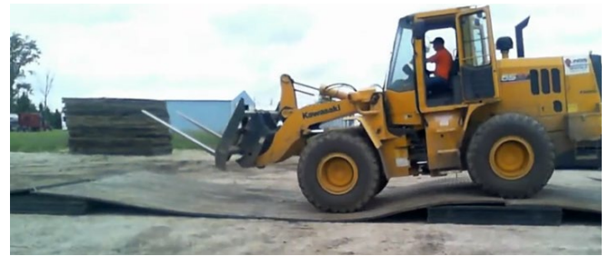
TuffTrak ground protection mats have a load bearing 330,693 lbs dependent on ground conditions.
